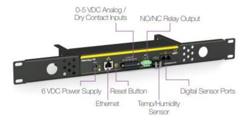
The Watchdog 100 is a self-contained unit with an on-board temperature/humidity/ dew point sensor. It has an input capacity of eight external sensors and relay output for triggering external devices, such as an auto-dialer.
